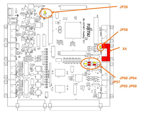
Figure 6-1: Jumper setting on starterkit SK-91F467D-208PFV
