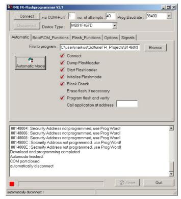
Figure 6-4: Successful Programming in Automatic Mode
