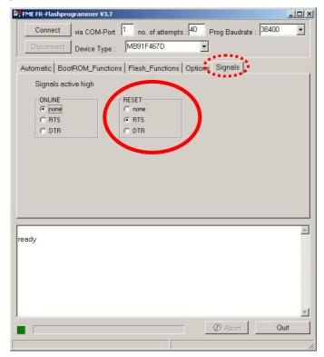
Figure 6-3: Reset Signal Settings
